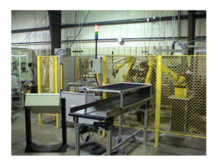
and bottom-side-up. In this manner, both sides of the part are flame etched, receive a gasket, and are allowed to cool. When finished, the second robot places a completed part on an outbound conveyor.
