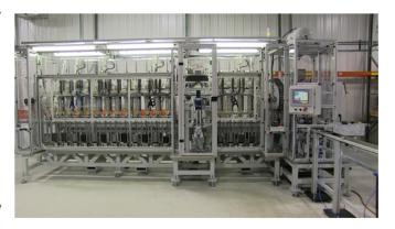
Mid-point and post-assembly measurements verify the thickness of the clutch packs using load-cells and LVDTs. This ensures that all packs are produced to the highest standard set forth by the client. With the goal of uninterrupted production, Flexible Automation Inc. integrated part magazines on either side of the machine, allowing for continuous production with minimal human interaction needed.
